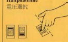
En If a voltage switch is located on the electronic circuit board of the controller, set it to the corresponding power supply (115 or 230 V).
